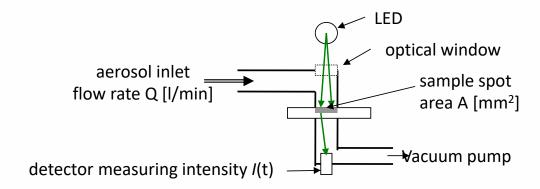
While loading the filter with particles the intensity I(t) and is measured and Attenuation is calculated by  $ATN = -ln(\tau)$
