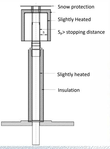
**Isokinetic Aerosol Sampling**
