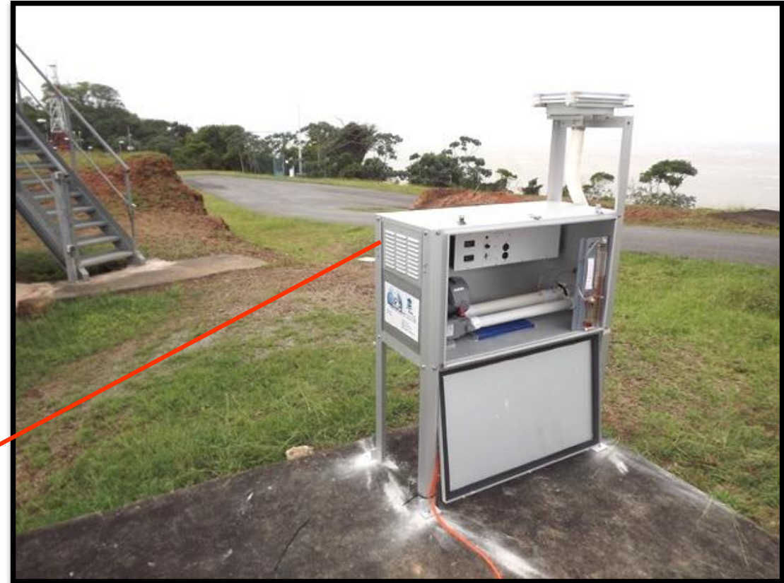
Photo of high volume air sampler in Cayenne. The same as used in previous UM global sampling activities.
